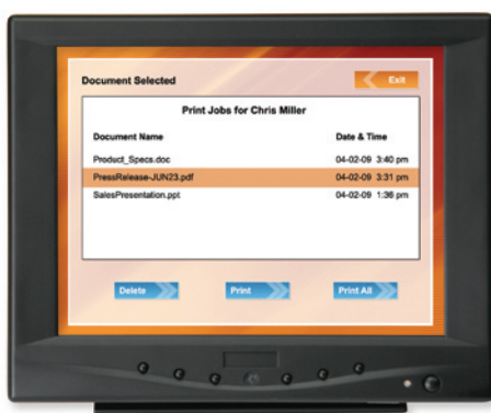
Employees use the PS150 touchscreen to select and release the jobs they need to print.
